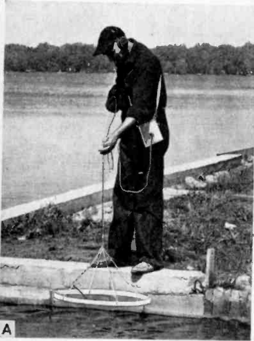
Working from a boat or dock the large loop finds lost outboard motors, cameras and even keys. A small loop wound on a plastic tumbler detects nails and pipes in the wall.
