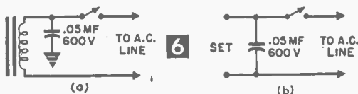
Suppressing a strong local station by connecting .05 mfd capacitor from one side of line to chassis ground for ac radio (a) and from set side of the switch to opposite side of line for AC-DC radio (b).
