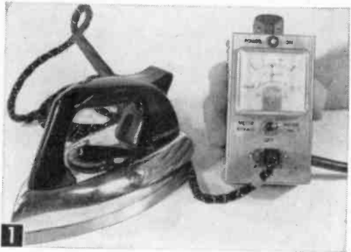
Just plug your appliance into the tester. An 8-ampere reading on the dial indicates normal operation of the iron, but an intermittent movement of the needle would indicate a faulty contact in the cord connector.
