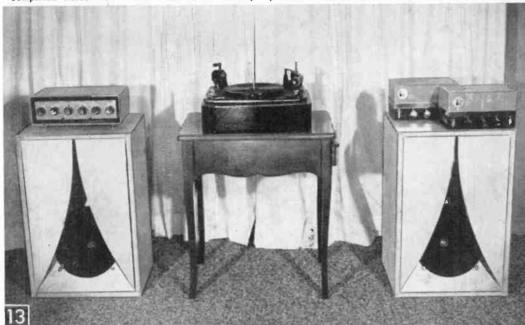
Without cabinet, the equipment looks like this: preamp over one speaker enclosure, amplifiers (to be remotely installed as in Fig. 2) over the other, record player. Tuner and tweeters not shown.
