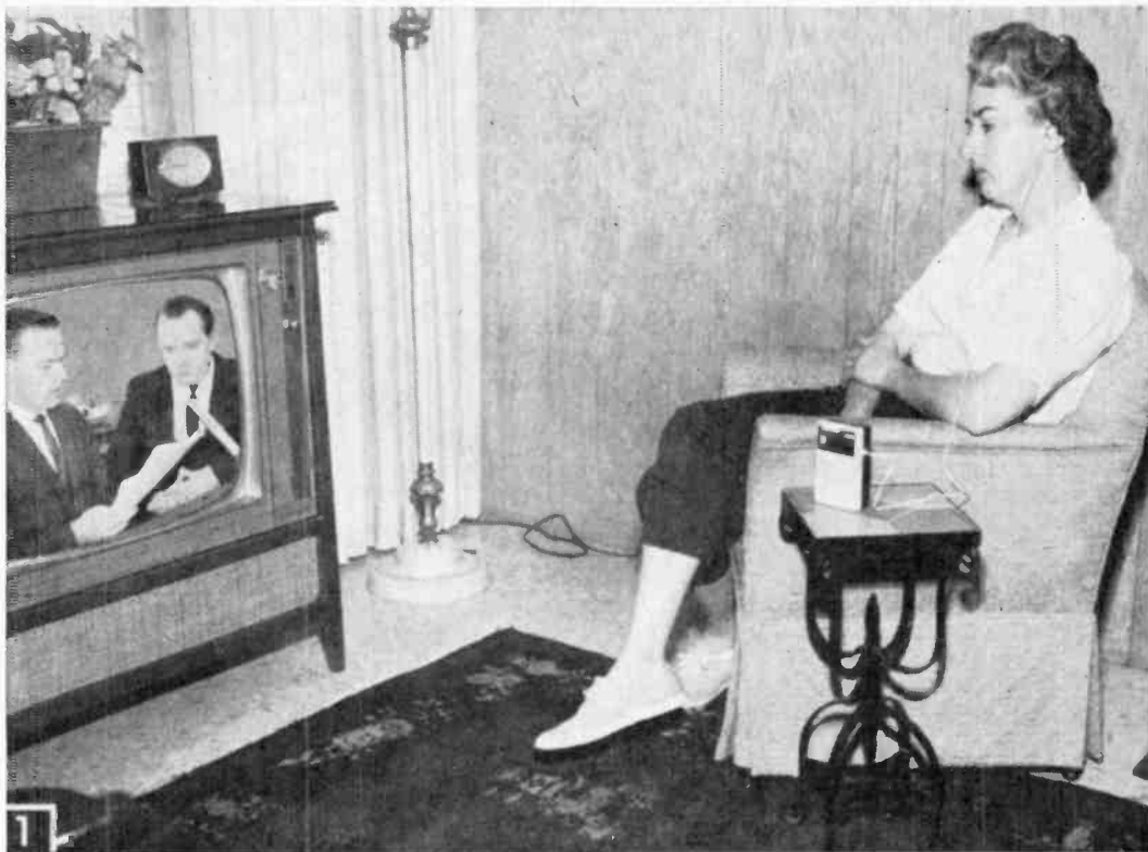
With TV speaker silent, the sound is picked up remotely by an earphone-equipped transistor radio.
