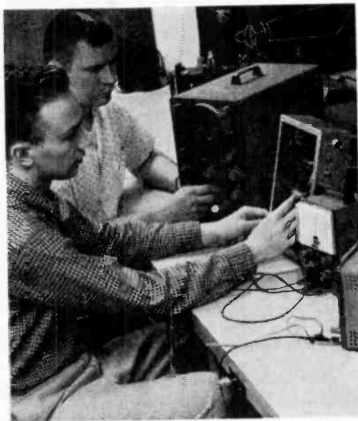
Station personnel design and maintain most of the equipment. These technicians are checking out a malfunctioning transmitter with an oscilloscope.
