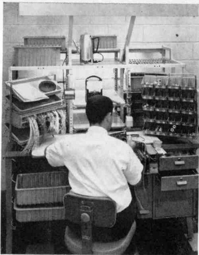
Here's a version of the Space Station as assembled by an electronic hobbyist. Note wire box at left, swivel parts bins, spools for solder and wire.
