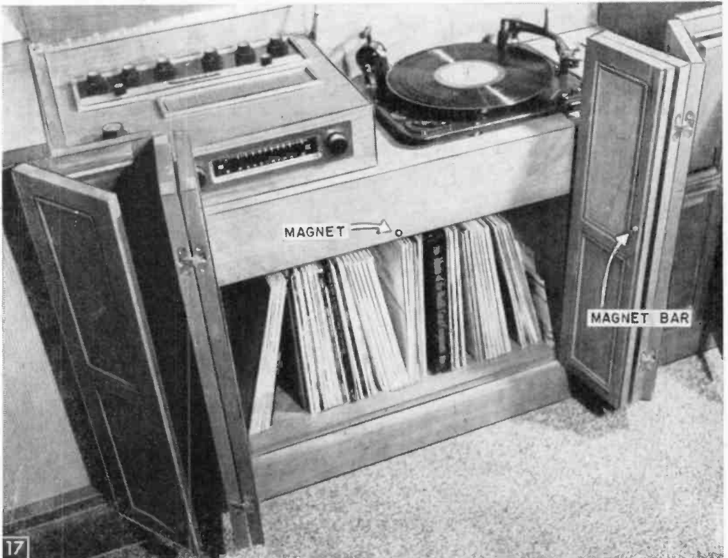
Completed control section and record compartment. Note tiny magnet recessed in front panel. Strong enough to hold doors closed, it releases with a slight pull.
