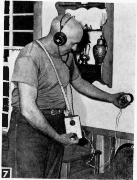
Working from a boat or dock the large loop finds lost outboard motors, cameras and even keys. A small loop wound on a plastic tumbler detects nails and pipes in the wall.
