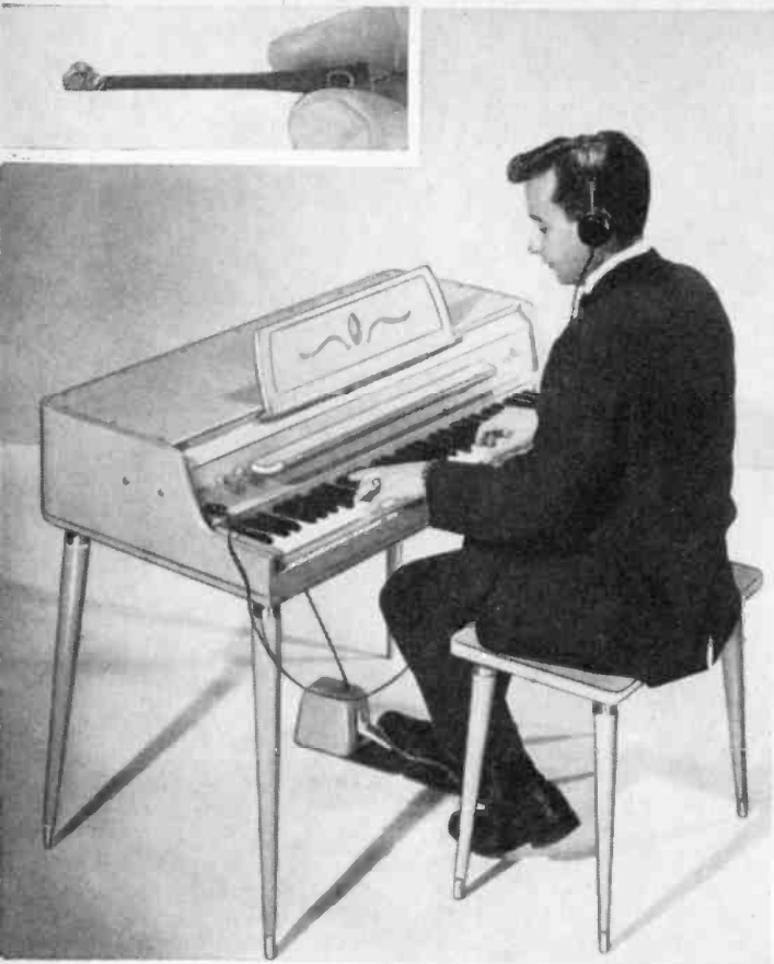
FIG. 1: This is the portable model Wurlitzer electronic piano. Amplifier and speakers are built-in. Foot pedal controls the sustain while keyboard knobs control volume and vibrato rheostats. Heart of electronic piano (left) is Swedish steel Sandvik reed . . . this one for a middle tone is about 2½ inches long. It bolts to the reed bar, hole at right for that purpose. Tip weight is ground or filed in reed pitch adjustment at factory.
