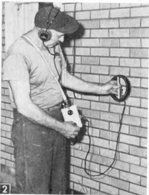
This small coil locates pipes buried in walls, floors, and concrete and can also be used to search for buried metal objects.
