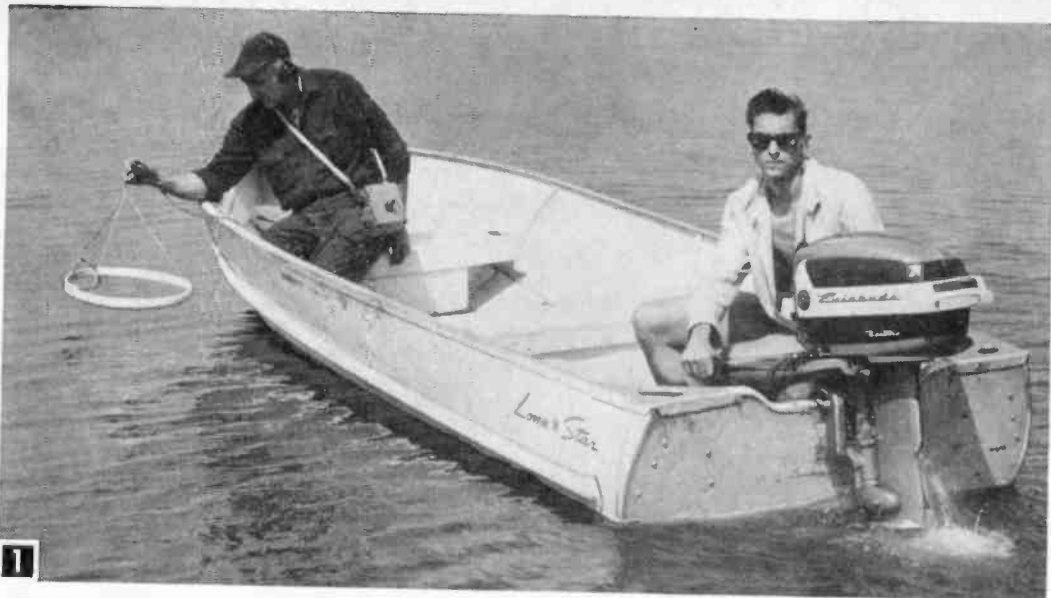
S&M Boat Designer Bill Jackson demonstrates search method. A 26-in. loop is wired into a 100-ft. cable made of lamp cord. When the coil approaches the metal object, a change in tone is heard.
