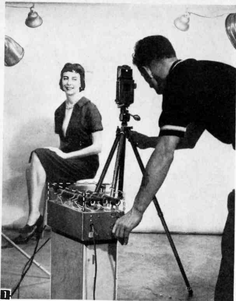
Cameraman shoots color portrait using studio booster. A combination of 50, 100 and 150 watt house lamps gives him well balanced main light, side lights and background lights.
